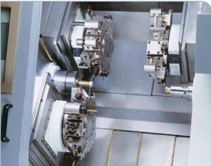
⚡ Up to 13 axes, 3-5/8” universal turn/mill center with 35 HP main-spindle, Fanuc 31i-T CNC control. 3-12 station turrets, and depending on model, live tooling, C-axis, 2-5/8” Y-axis travel and sub spindle
